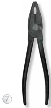
7 In a chamber hardening kiln, the pliers are hardened in a protective gas atmosphere, quenched in oil and finally annealed. The design of the hardening kiln ensures that the process gases are uniformly distributed, which has a positive effect on the desired material properties.
