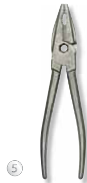
5 The joint faces are precision milled. The pliers head takes on its final form.
