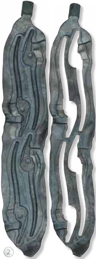
2 Hot forged in the double forging die. The excess burr is removed under an eccentric press.
