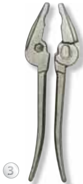
3 The blanks are "normalised" to obtain an even finer-grain, more uniform structure with optimum strength. After descaling, the blanks are calibrated for the following work steps.
