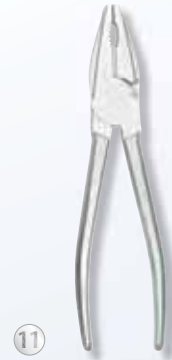
11 Nickel-plated and matt-chrome-plated to prevent dazzle. The electrolytically deposited nickel coating provides the corrosion protection. The electroplated chrome improves the look and gives the pliers a perfect finish.
