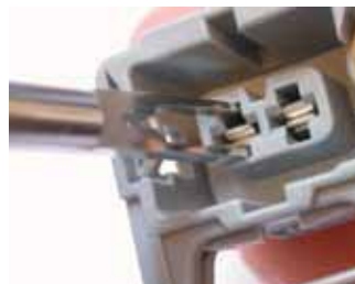
Insert flat pin tool into unlocking channel and release pin
