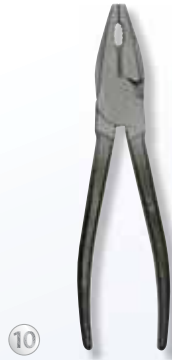
10 The surface is cleaned by sand blasting. The removal of scale and grease is necessary for the follow-on electroplating process.
