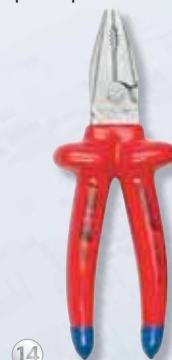
14 The plastic coating on the handles is built up by multiple dipping in liquid immersion compound.
