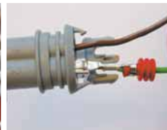
Remove released pin from casing
