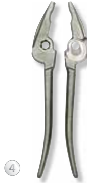
4 The head is machined in a CNC-controlled machining centre. The rivet hole is drilled and counter-bored. The joint clearance and the outer contour are milled. The geometry of the joint area and the coarse and fine toothing are broached.
