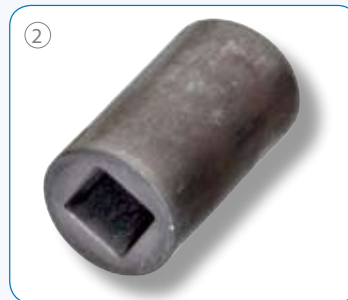
Hot forged in the forging press.
